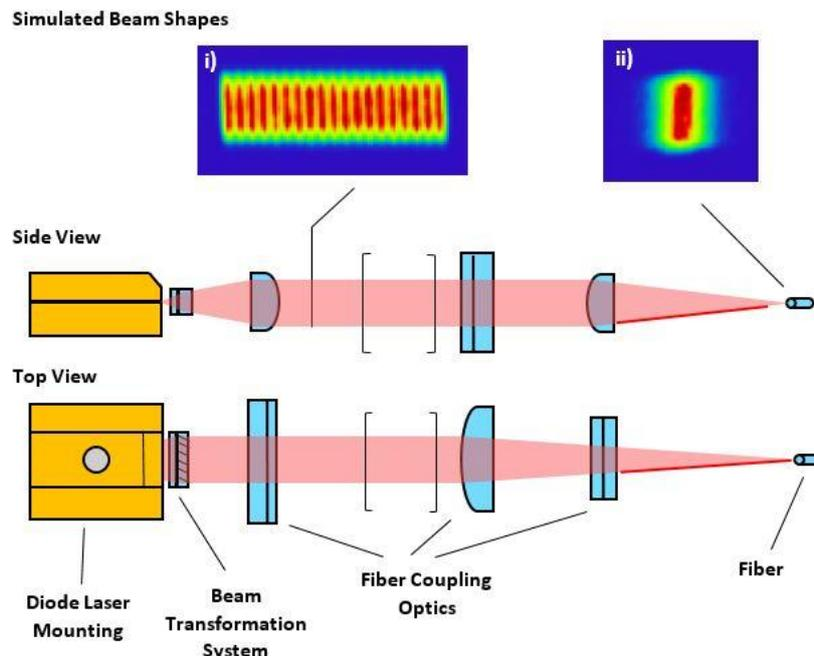
Figure 6. Fiber coupling optical system and the simulated beam profiles along the beam path i) Collimated beam profile after the BTS+SAC combination and ii) beam waist at the fiber facet.
