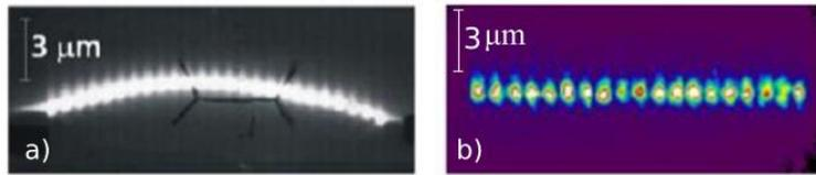
Figure 4. a) Enlarged picture of a soldered diode laser bar with a ‘smile’ of approx. 2  $\mu\text{m}$ . Image taken from Ref. 8. b) Enlarged picture of a diode laser bar mounted with *Clamping™*, showing a smile under 0,1  $\mu\text{m}$ .
