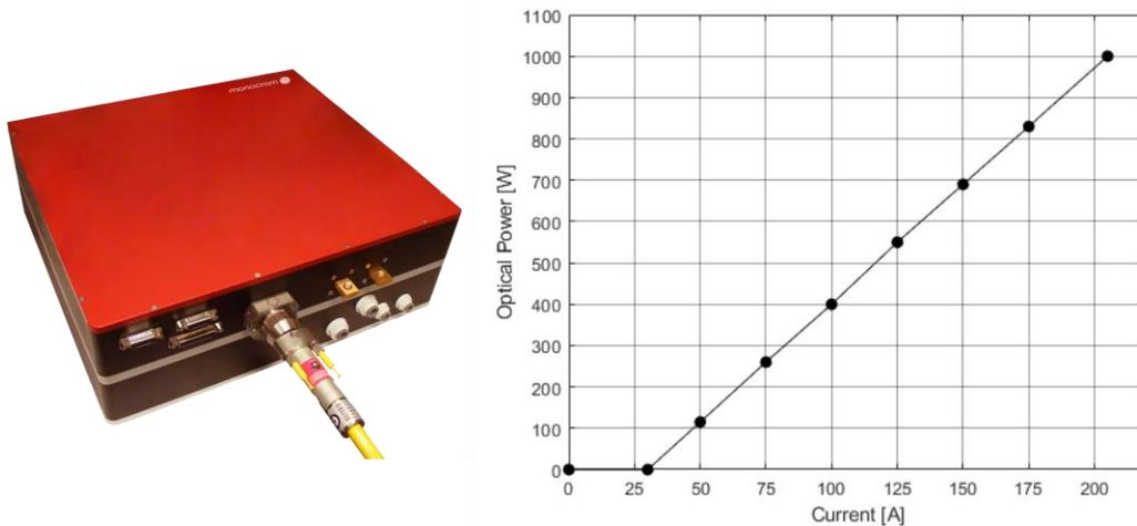
Figure 8. Monocrom 1 kW cw fiber-coupled module (left) and the corresponding power vs current diagram (right).
