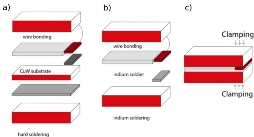
Figure 3. Schematic view for laser bar mounting with a) hard soldering with gold-tin, b) soft soldering with indium, and c) *Clamping<sup>TM</sup>*.
