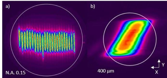
Figure 7. a) Focused beam far field. The circle represents a numerical aperture of 0.15. b) Magnified image of the focused beam at the fiber face. The circle has a diameter of 400 μm.
