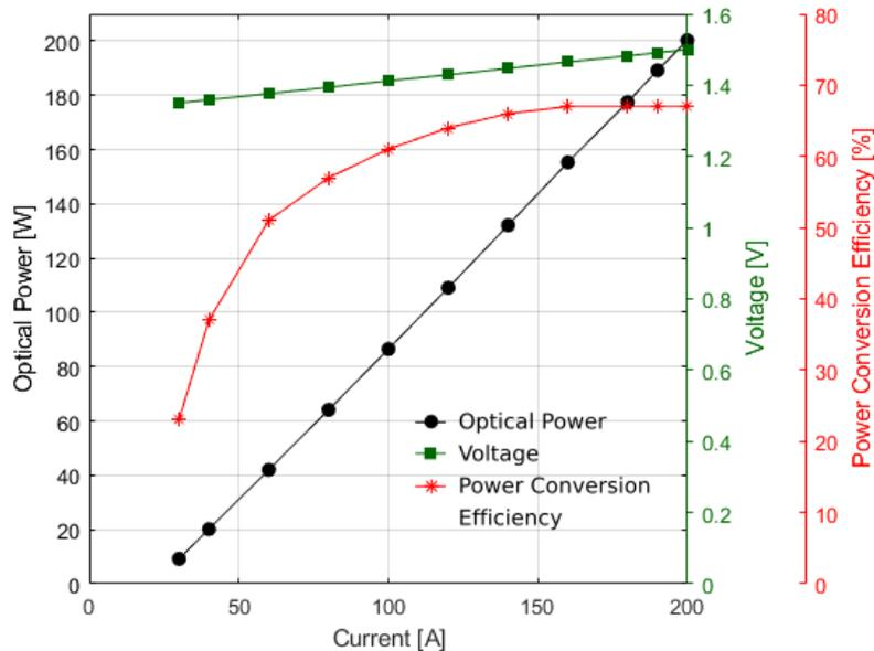
Figure 5. Dependence on driving current of optical power, voltage and power conversion efficiency of the single diode laser bar module (diode laser bar mounted using *Clamping™*).
